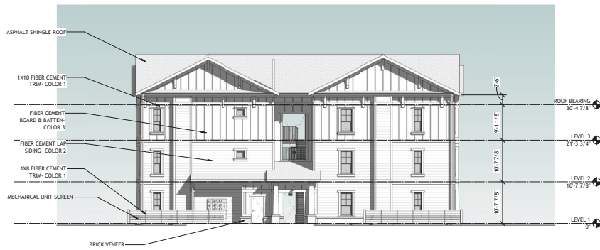
2 SD PRESENTATION- ELEVATION- BLDG. TYPE C LEFT A3-030 3/32" = 1'-0"
