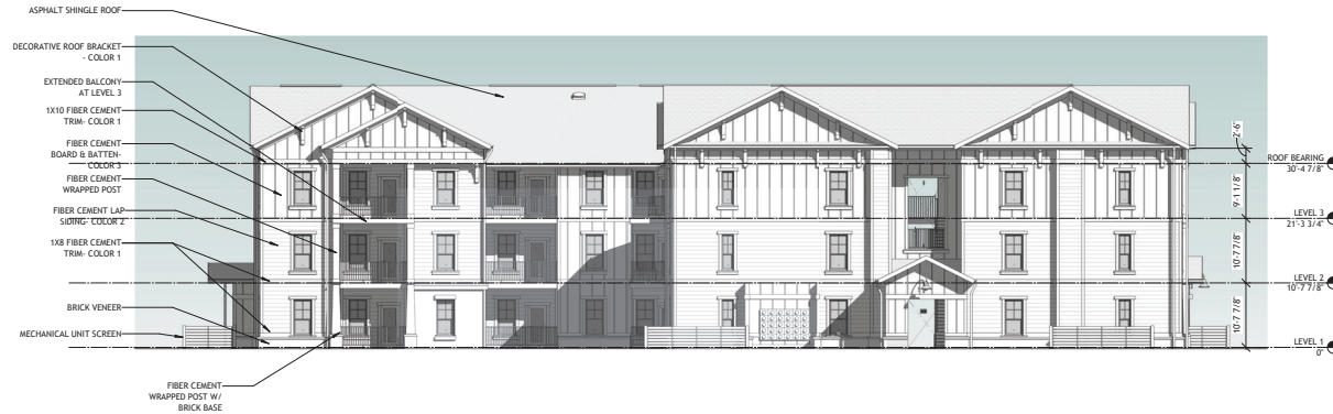
1 SD PRESENTATION-ELEVATION-BLDG. TYPE B REAR A3-021 3/32" = 1'-0"
