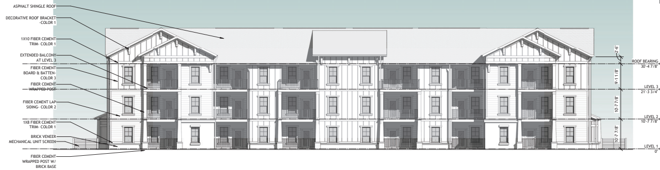
1 SD PRESENTATION- ELEVATION- BLDG. TYPE C FRONT A3-030 3/32" = 1'-0"
