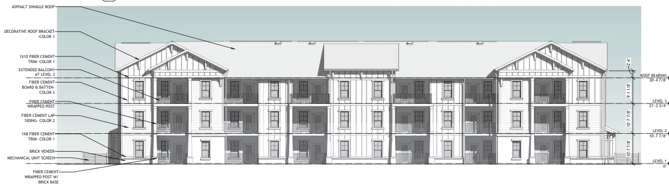
3 SD PRESENTATION - ELEVATION - BLDG. TYPE C REAR A3-030 3/32" = 1'-0"
