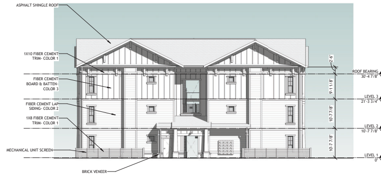
4 SD PRESENTATION- ELEVATION- BLDG TYPE C RIGHT A3-030 3/32" = 1'-0"
