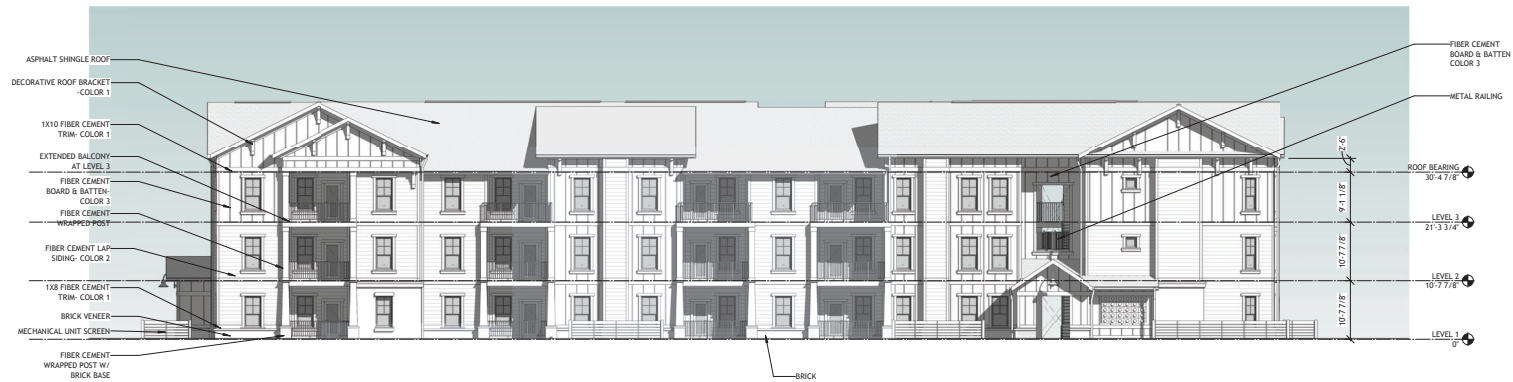
1 SD PRESENTATION-ELEVATION- BLDG. TYPE D FRONT A3-040 3/32" = 1'-0"
