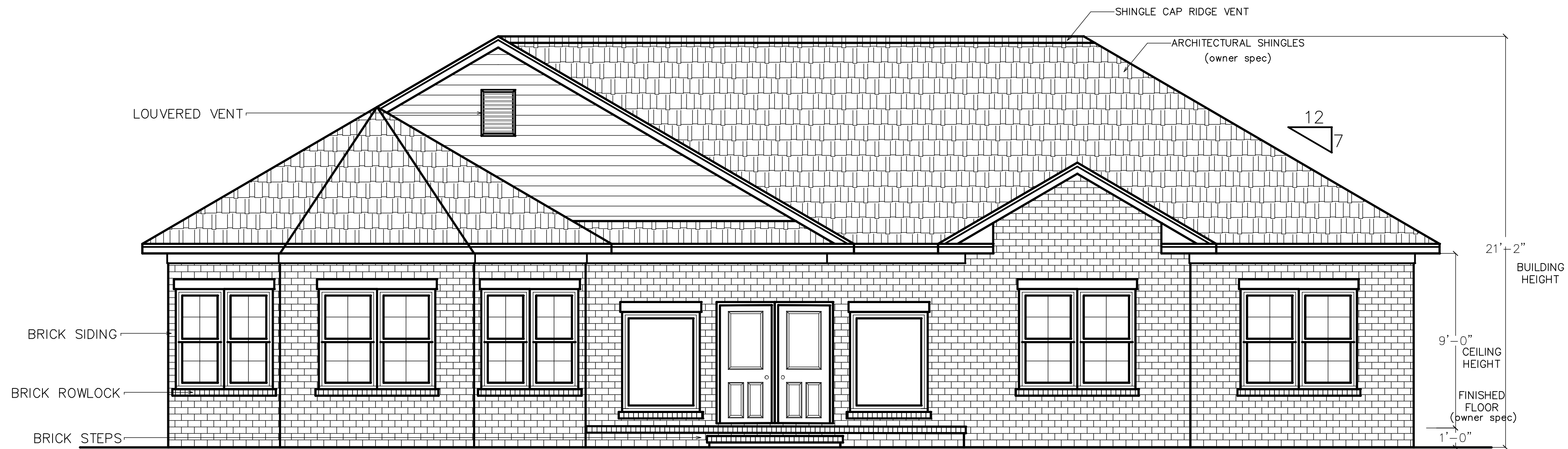
PROPOSED FRONT ELEVATION SCALE=1/4"=1'-0"
